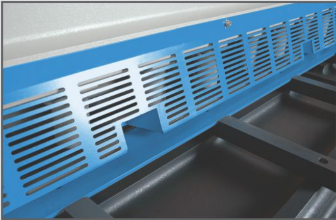
Hand safety guard with hand gaps for handling small sheets.
